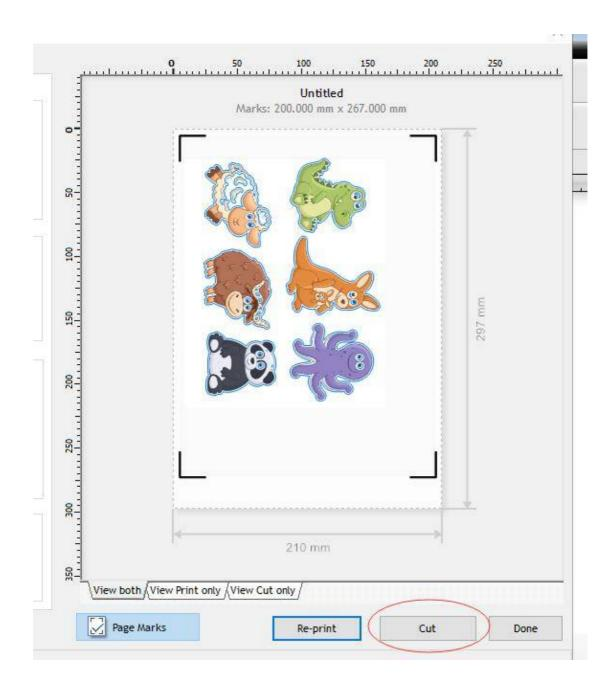
Load the printout onto cutter, and take care of the blade or pen setting position. (inside the first mark)
